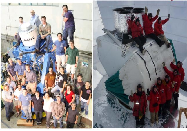
BICEP1 (2006 – 2008) 30cm refractor 96 NTD bolometers (same kind as Planck) Best published limits on r from B-modes – r<0.72 BICEP2 (2010 – 2012) Same optics as BICEP1 500 TES bolometers at 150 GHz 10x faster than BICEP1 Keck-Array (2011 – 2015) 5 BICEP2 like receivers 2500 TES bolometers 5x faster than BICEP2
