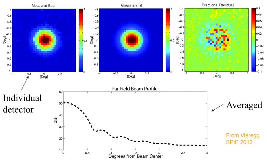
• Using chopped thermal source (unpolarized)
